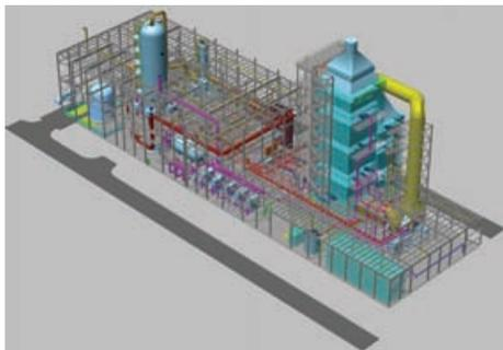
Figure 3: 3D Model of SaskPower Carbon Capture Plant
